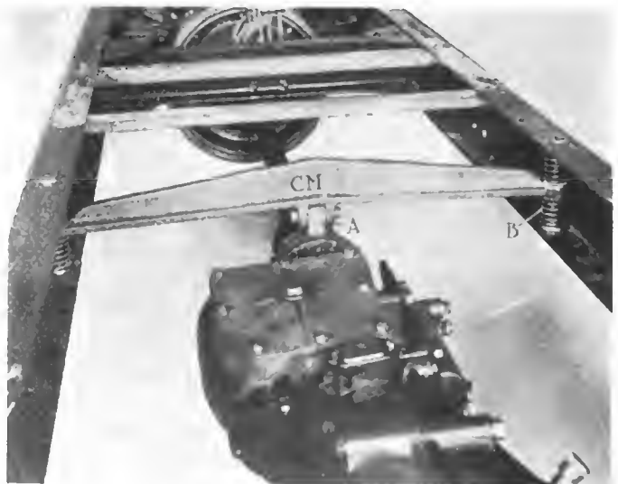
Wilson 1½-ton truck, showing unique mounting of front end of gearset. The cross member C M holds it up in position through connection A. This member is supported at either end in the frame through the spring buffers B. Thus, the vibration and road shocks are not transmitted to the gearset and jackshaft. By removing the pin at B and disconnecting the propeller shaft, the entire gearbox and jackshaft may be swung downward for inspection or adjustment
